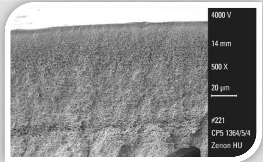
Cross section of UF membrane magnified 500 times.
